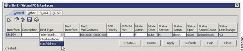
Figure D-6 Changing The Bind Type From Interface to Mac Address
